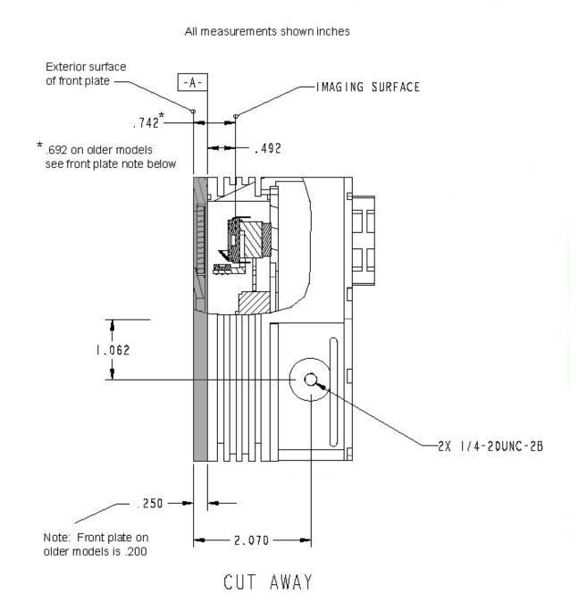
The camera front plate (shown in gray) was made thicker in recent models. It is easy to measure from the outside of the camera. The front plate in this drawing does not include the "D" block with T-thread ring which is approximately .270" thick.
